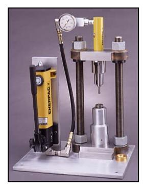
The Manual Tablet Compression Machine, Model MTCM-I, is designed for compaction of powders into tablets one at a time.
