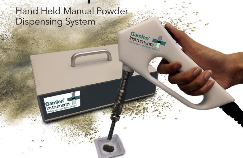
The GamPette<sup>™</sup> is a hand held powder pipette that accurately dispenses solids. It comprises of a dispensing handle and a controller unit. Tip sizes are available to accommodate a wide range of powder volumes. Powder is drawn into the pipette tip in the handle under vacuum, and then expelled under light positive pressure.
