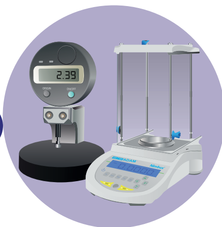
MEASURE THE TABLET Electronic Micrometer and Balance
