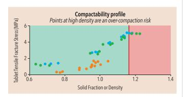
Compactability is the effect of solid fraction on tablet strength. We have to balance these properties to have strong tablets without over-compation.
