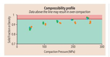
Compressibility describes how tablet solid fraction changes with compaction pressure. High solid fraction values hinder water penetration reducing dissolution rate.
