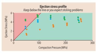
Ejection stress is a measure of how well lubricated the formulation is. Poor lubrication results in tablet defects picking, sticking and capping.
