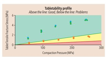
Tabletability is the dependence of tablet strength on compaction pressure. We maximise tabletability to produce a robust tablet which will withstand handling.
