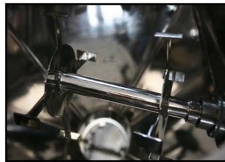
GlobePharma's new MAXIBLEND® 1-2 PILOT-SCALE BLENDER is an all stainless-steel self-contained tumble blender for use with powders.
